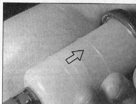
6.4 Ensure arrow (highlighted) on filter body is pointing towards the pump
