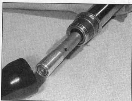
3.8a Fit the damper rod seat to end of rod lubricate guide bush and insert stanchion assembly into lower leg
