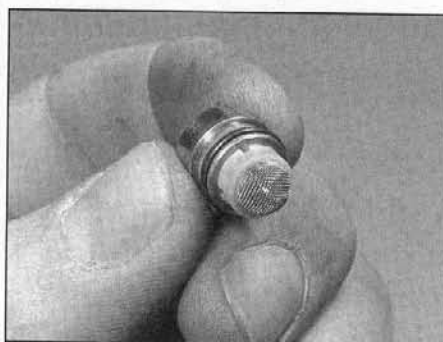
8.3e Clean needle valve seat filter and renew the O-ring
