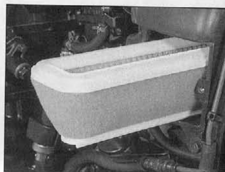
14.1c ... and withdraw the air filter element
