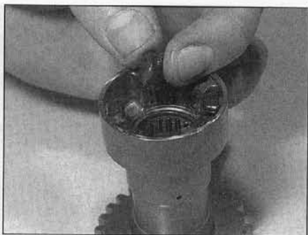
32.4a Use grease to hold the cush drive rubbers in position
