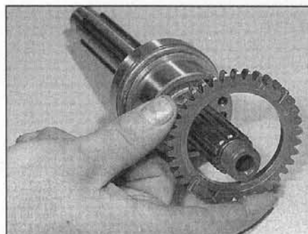
31.7d ... and the oil pump drive gear with its dogs facing away from the thrust washers
