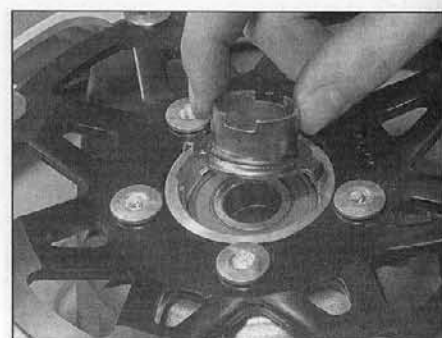
6.5d On the front wheel locate speedometer drive plate with slots in hub . . .
