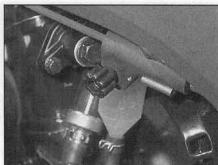
7.9 Idle speed adjuster is situated on left-hand side carburettors - ZX1100 C/D shown
