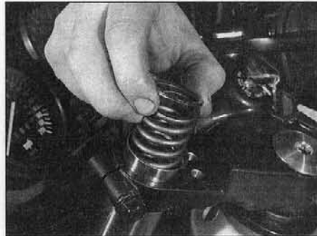
3.10c On ZX1100 D models install plain washer on top of fork spring . . .
