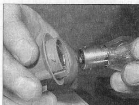
21.5b Note offset pins on bulb to prevent incorrect installation
