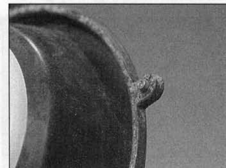
8.2e On ZX1000 B and ZX1100 C/D models note air jet set in diaphragm or carburettor casting
