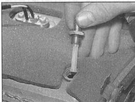
17.2 On ZX1100 C/D models fuel filter is separate from the fuel tap and is a screw fit in the tank
