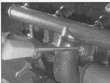
7.2a Cooling system hoses are secured with clamps ...
