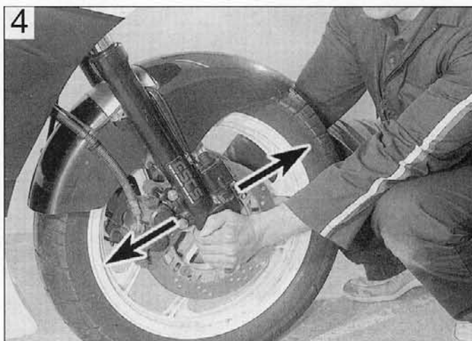
Checking the steering head bearings for freeplay
