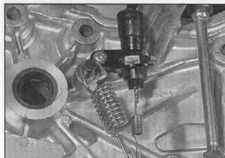
8.15 On ZX900 models remove the footrest bracket to adjust the brake pedal and stop lamp switch
