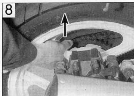
Checking for rear suspension linkage play
