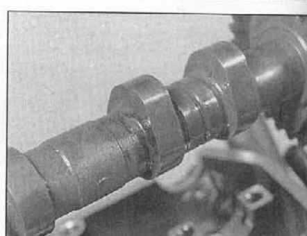
21.1 Examine cam lobes for signs of scoring
