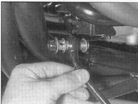
4.4a Remove all union bolts which secure the oil cooler hoses to the engine unit.
