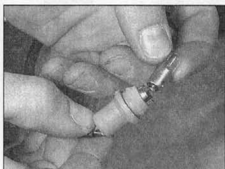
21.4b . . . bulb is a bayonet fit in its holder
