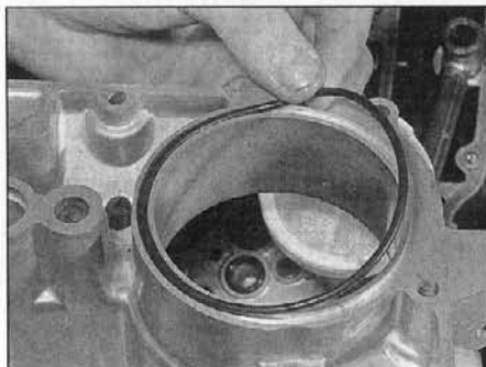
39.3c Fit a new O-ring around the oil filter chamber in the sump ...
