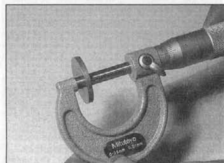
Tappet shims are measured with a micrometer
