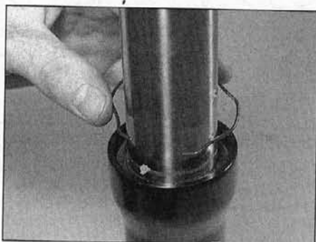
3.9b Secure the seal with the circlip
