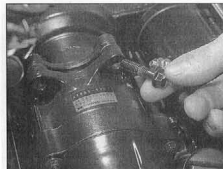
38.2b Refit alternator - apply threadlocking compound to its bolts and tighten to specified torque setting
