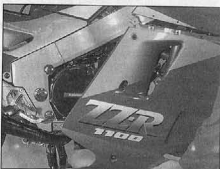
23.17g Offer up the lower fairing sections ...
