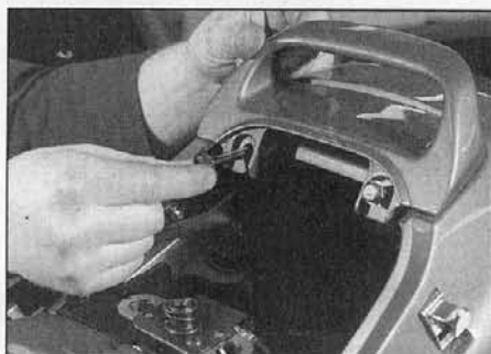
25.2 Grab rail is retained by two bolts
