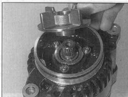
6.11 Stator coil is retained by three screws situated behind drive coupling
