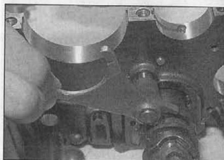
34.1b Position the left-hand selector fork and insert the selector fork shaft until it engages with the fork . . .
