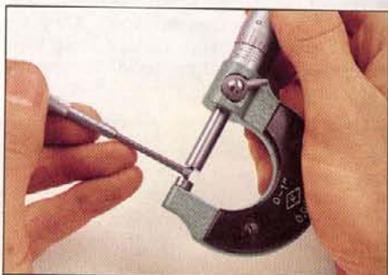
3.10 ... then measure the gauge with a micrometer
