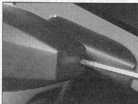
21.6a On ZX900 models release screw from the back of the lamp . . .
