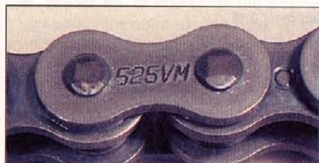
8.10 Typical chain size and type marking
