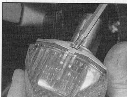
21.6b . . . remove lens assembly and slacken two screws which secure lens to the bulbholder
