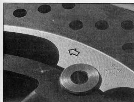
8.3 Where discs show a stamped arrow ensure this faces in normal direction of wheel rotation
