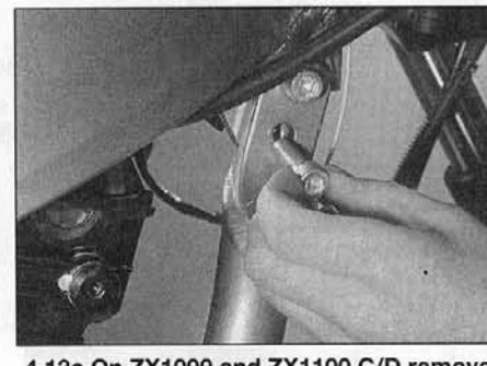
4.13a On ZX1000 and ZX1100 C/D remove the engine front and frame cradle mounting bolts ...
