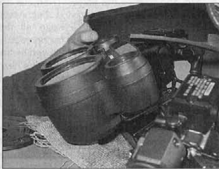
23.3 Cover the fuel tank with a clean rag and rest the instrument panel on the tank
