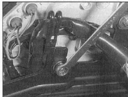
20.3 Instrument are retained to mounting bracket by two nuts
