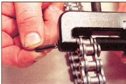
8.2 ... withdraw the pin, remove the tool ...
