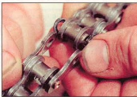
8.3 ... and separate the chain link
