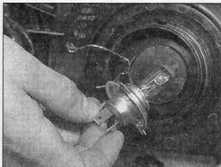
21.3a Fit the bulb to the headlamp unit . . .
