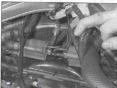
6.1a HT coil location - ZX1000 B and ZX1100 C/D models
