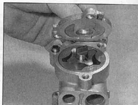
17.4c Ensure dowel is in position before refitting end cover
