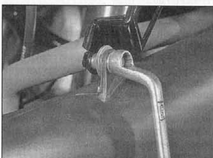
46.8 On ZX1100 C/D models do not omit shouldered spacer from behind front air filter housing mounting bolt
