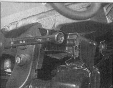
5.4a Remove the radiator mounting bolts . . .
