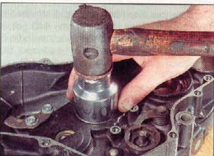
5.2 Using a large socket against the bearing's outer race
