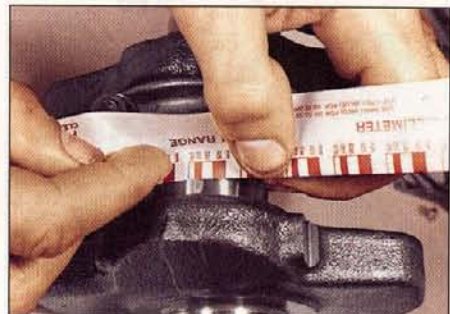
3.16 Measuring the width of the crushed Plastigauge
