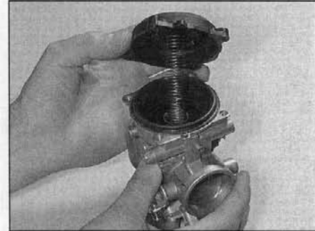
8.2a Remove four screws and lift off top cover. Withdraw return spring ...
