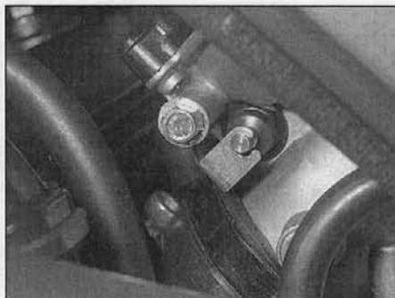
7.6 Choke mechanism is on the left-hand side of carburettor bank - plunger must operate smoothly
