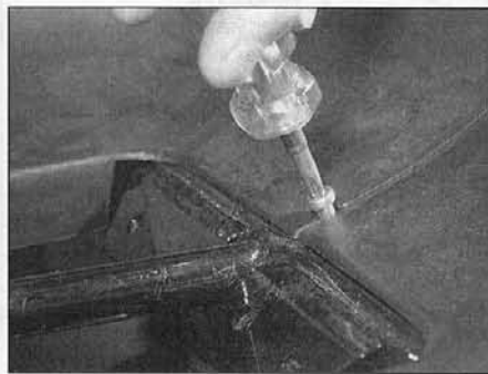
23.4a Slacken the upper inner fairing retaining screws and carefully remove the inner fairing sections
