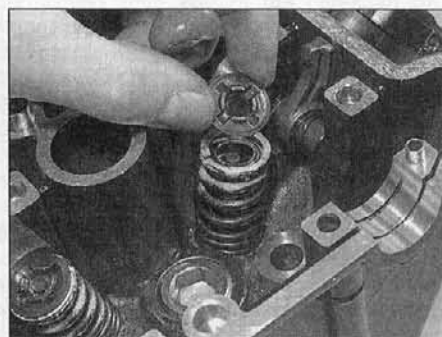
23.14e ... followed by the spring retaining collar
