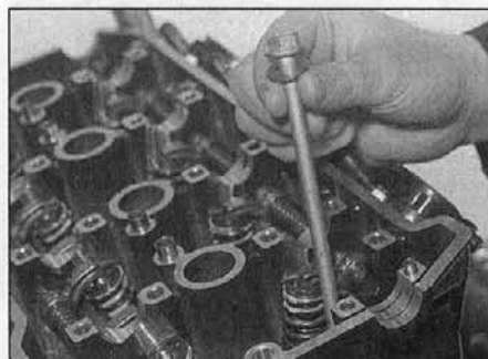
42.6b Flat-headed cylinder head bolts are fitted to the four outer holes ...
