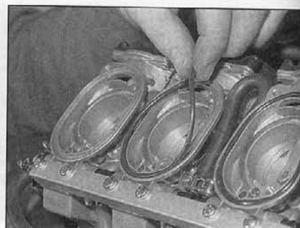
7.10 On ZX1100 C/D models do not omit O-rings from the carburettors
