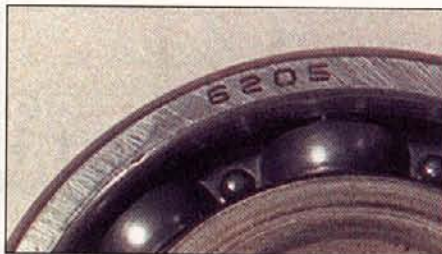
5.16 Typical bearing marking
