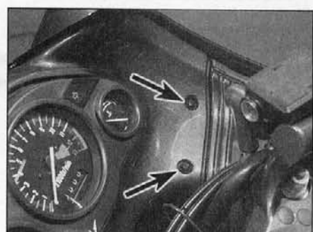
23.24 Instrument panel cover is retained by two screws (arrows) on each side
