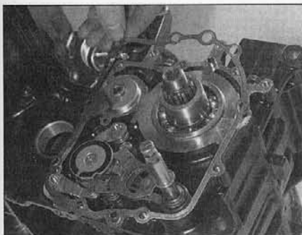
37.3a Refit dowels to the crankcase and position a new gasket over them
