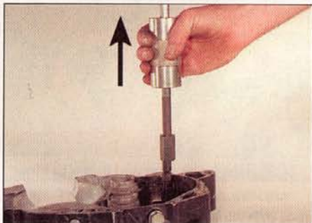
5.7 . . . attach the slide hammer to the bearing puller
