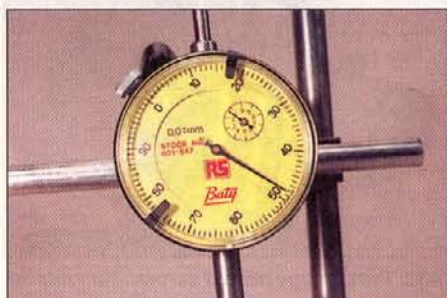
3.17 Dial gauge reading of 1.48 mm
