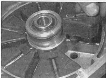
Cush drive rubbers dampen out transmission shocks
