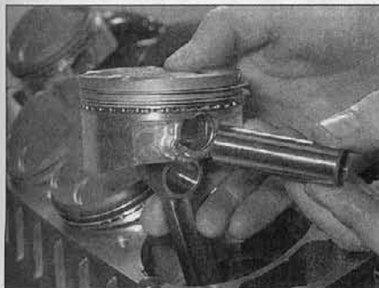
42.2b Insert the gudgeon pin into the piston ...
