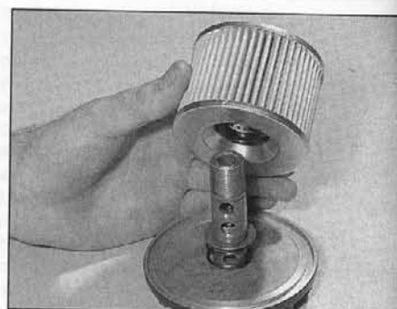
13.3c ... and carefully screw on the new element
