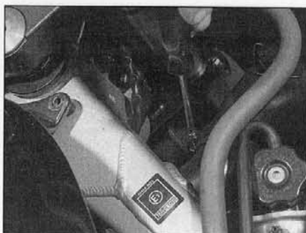
23.28b . . . and slacken the screw on each air intake duct clamp
