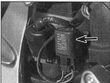
19.1a On ZX1100 C models turn signal relay is situated next to starter relay
