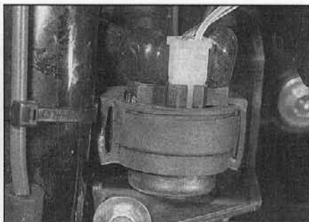
8.3b Starter relay location - ZX900 models
