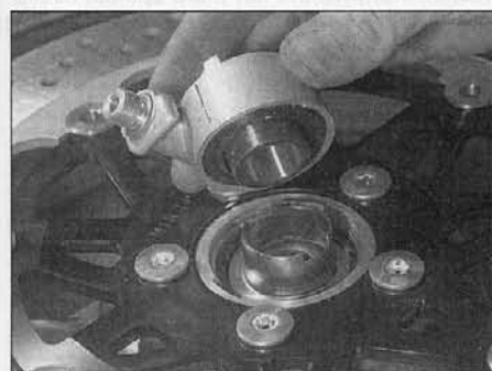
3.1a Refit speedometer gearbox ensuring that it is correctly located ...
