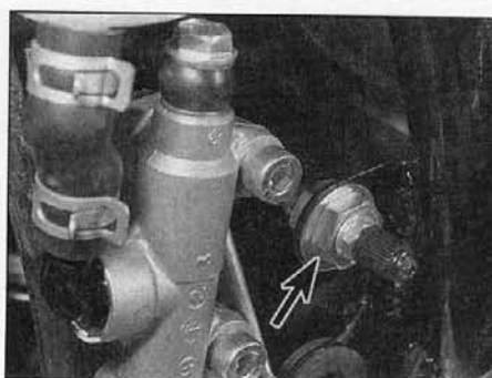
11.2b Remove the air valve mounting nut
