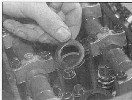
45.11b Do not omit cylinder head cover dowels
