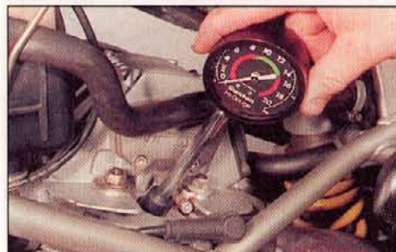
3.20 Using a rubber-cone type cylinder compression gauge
