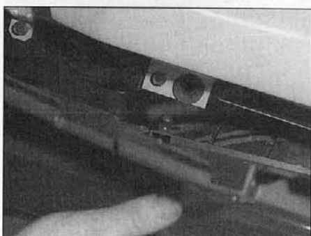
25.5a Ensure that panel stub engages grommet on refitting
