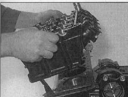
42.6a ... and lower the cylinder head assembly onto the block
