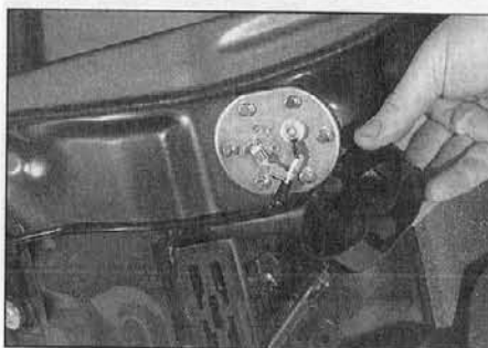
22.1 Fuel level sender unit is retained by six screws
