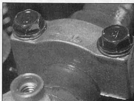
45.5b ... and install the bearing caps using the arrows and numbers cast into the top surface
