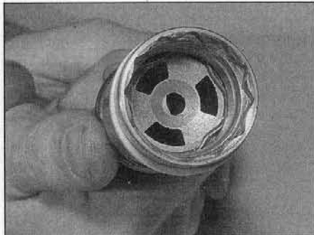
3.10b . . . and ensure the damping adjuster rod engages correctly with damper rod
