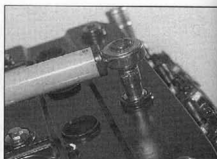
45.11d . . . and tighten its retaining bolts evenly and progressively to the specified torque setting
