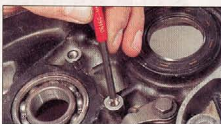
2.30 ... break off the tang when complete
