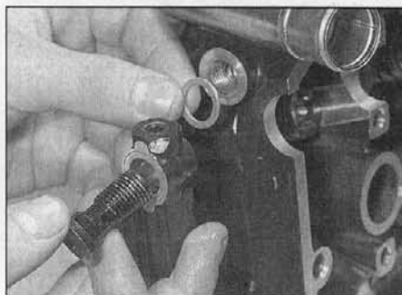
45.1b ... and use a new sealing washer when refitting oil pipe union
