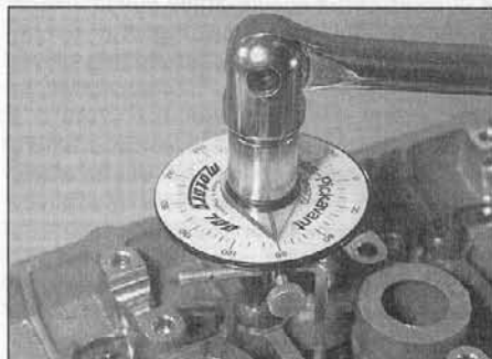
Angle-tightening cylinder head bolts
