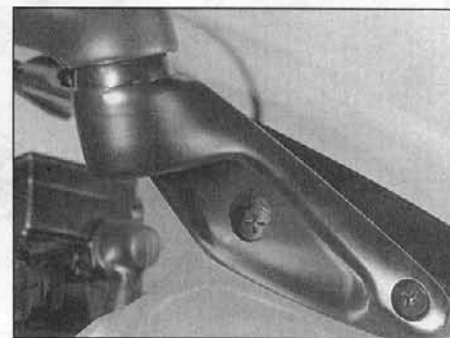
23.4b Remove the rear view mirror mounting screws ...
