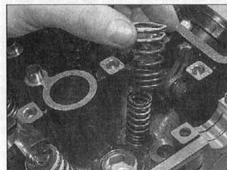
23.14d Refit the valve springs, ensuring that their closer-pitched coils are at the bottom ...
