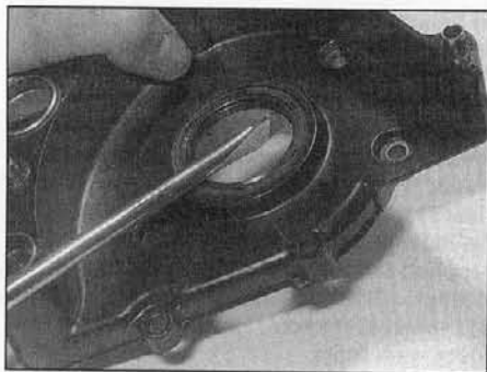
20.4a Carefully lever out old oil seals using a flat-bladed screwdriver . . .
