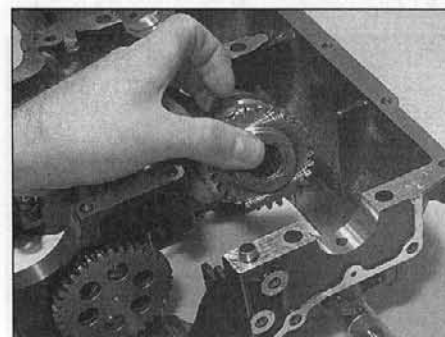
34.3a Position the balancer weight assembly in the casing and refit the shaft
