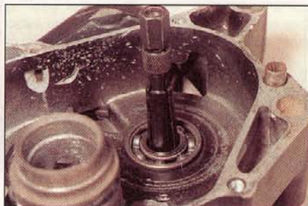
5.6 Expand the bearing puller so that it locks behind the bearing . . .
