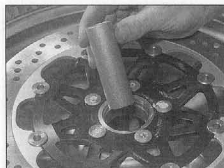
6.5b . . . then invert the wheel and insert central spacer
