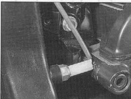
12.7 Fan switch is situated on the left-hand side of the radiator
