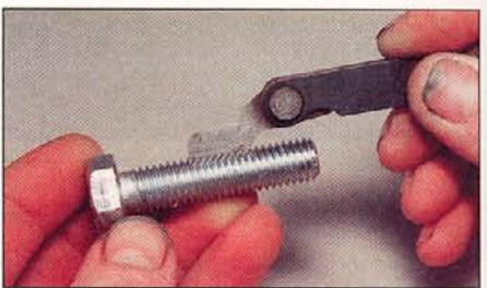
2.12 Using a thread gauge to measure pitch
