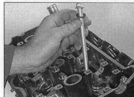
42.6c ... and tapered-headed bolts are fitted to the six inner holes
