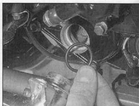
7.2c ... and sealed with O-rings
