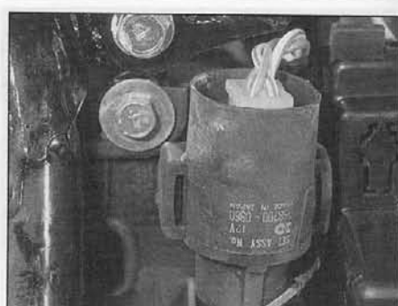
12.6 Fan relay is situated beside the junction box - ZX900
