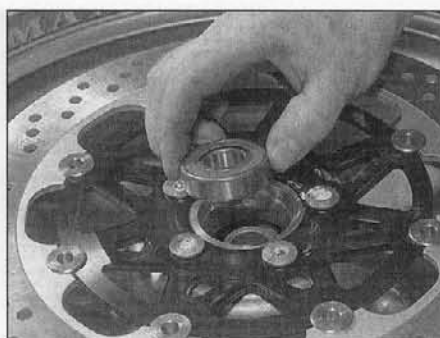
6.5c Grease the cavity and fit the second bearing
