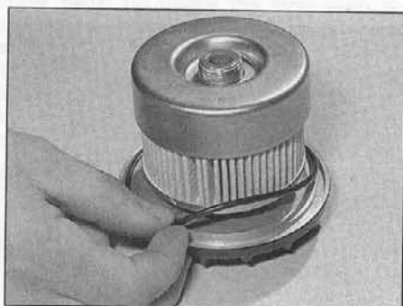
13.3d Fit the baffle plate over the element and a new O-ring to the cover ...
