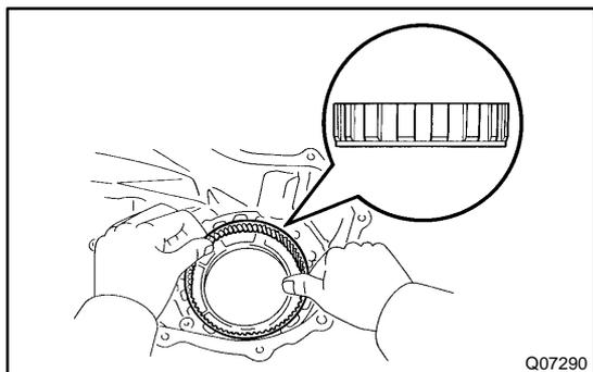
(c) Remove the planetary ring gear.
