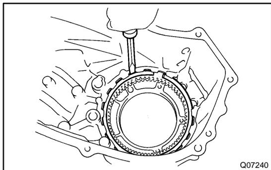
**32. REMOVE PLANETARY RING GEAR**
