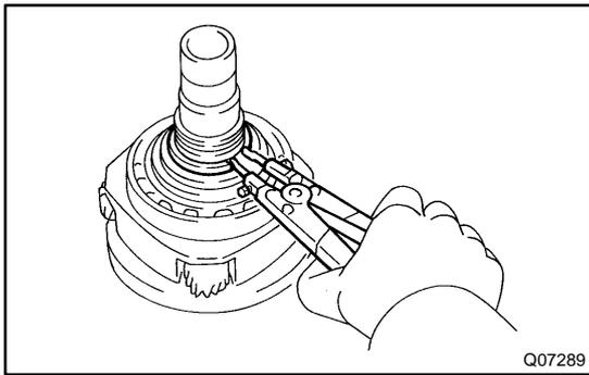
**30. REMOVE INPUT SHAFT STOPPER AND THRUST BEARING**
