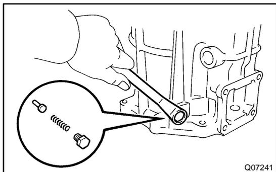
(b) Remove the plug, spring and pin.
