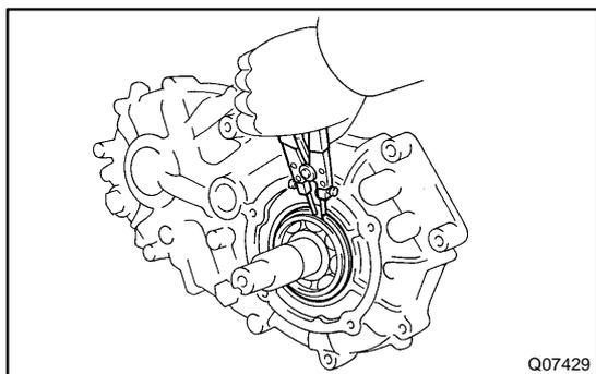
**21. REMOVE REAR OUTPUT SHAFT, DRIVEN SPROCKET AND CHAIN**
