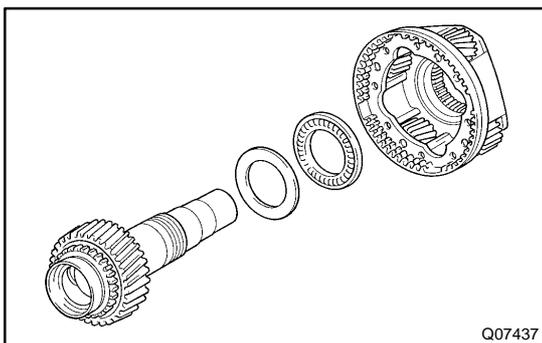
**31. REMOVE INPUT SHAFT, THRUST NEEDLE ROLLER BEARING AND THRUST RACE**
