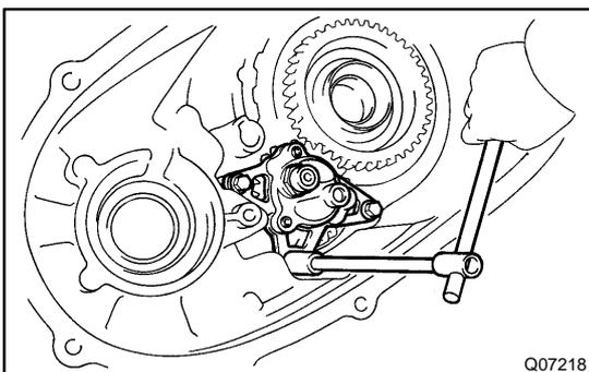
**24. REMOVE SEPARATOR WITH OIL STRAINER AND MAGNET**
