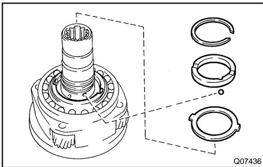
(b) Remove the input gear stopper, thrust washer and ball.
