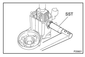
(2) Using SST, tighten the nuts to the specified torque.SST 09810–38140
