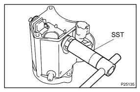
(c) Remove the terminal kit parts.
