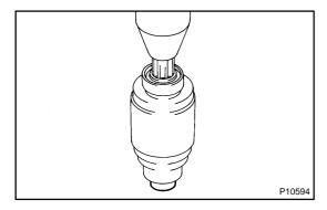
(b) Using a press, press in a new bearing.
