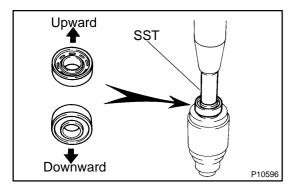
(b) Using SST and a press, press in a new bearing. **NOTICE:**
