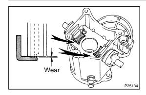
(b) Using vernier calipers, measure the contact plate for depth of wear.
