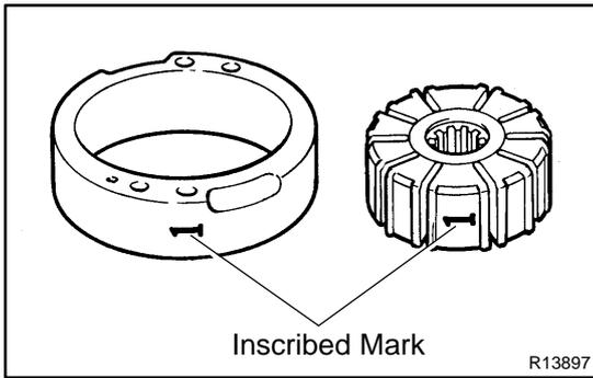
If it is more than the maximum, replace the plate and/or rotor with one having the same mark stamped on the cam ring.
