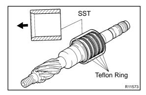
(e) Carefully slide the tapered end of SST over the teflon rings until the rings fit to the steering rack.
