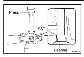
(b) Using SST, press out the bearing from the rack housing. SST 09950–60010 (09951–00260), 09950–70010 (09951–07200)
