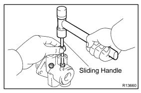
(b) Using a plastic hammer and sliding handle, lightly tap in 2 new union seats.
