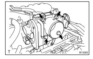
(b) Install the throttle body with the 2 bolts and 2 nuts.
