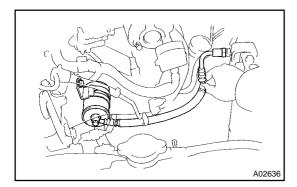
(f) Check that there is pressure in the inlet hose from the fuel filter.
