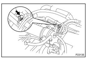
Remove the union bolt and 2 gaskets, and disconnect the (c) fuel inlet pipe from the delivery pipe.
