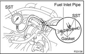
(d) Install the fuel inlet pipe and SST (pressure gauge) to the delivery pipe with the 3 gaskets and SST (union bolt).
