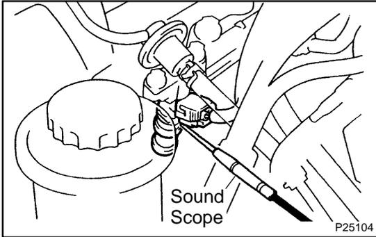
(b) Using a sound scope, check for injector operating noise.
