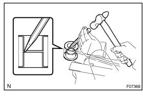
(c) Using a chisel and hammer, tap out the outer tubes.
