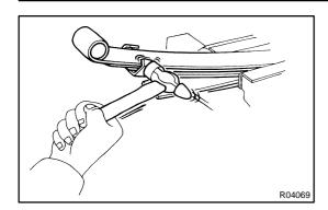
(e) Bend the spring clip.Using a hammer, bend the spring clip into the position.
