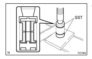
(d) Using SST and a press, install 2 new bushings. SST 09710–28012 (09710–07062), 09710–30041 (09710–03211)
