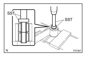
(b) Using SST and a press, press out the both inner tubes and rubber parts of the bushings.
