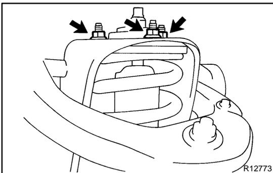
3. REMOVE SHOCK ABSORBER WITH COIL SPRING
