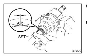
(b) Make sure that the boots are not stretched or contracted when the drive shaft is at standard length.
