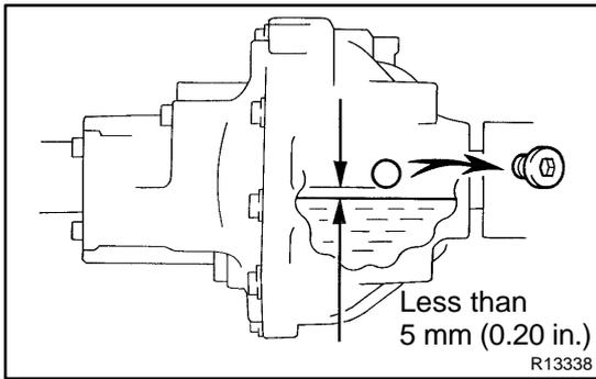
12. **FILL DIFFERENTIAL WITH HYPOID GEAR OIL**
