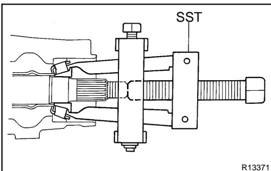
5. REMOVE REAR BEARING AND BEARING SPACER
