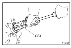
(b) Remove the oil seal.
