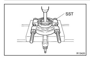
(2) Using SST, a brass bar and press, remove the bearing.
