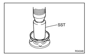
(b) Using SST and a press, install a new dust deflector. SST 09636–20010
