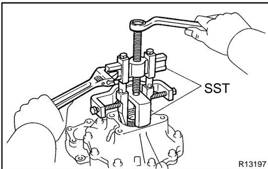
**9. REMOVE INTERMEDIATE SHAFT NO. 1**
