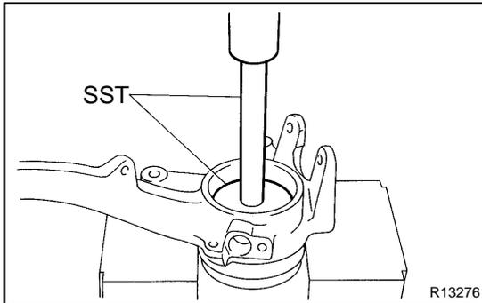
(b) Using SST and a press, remove the bearing from the steering knuckle.
