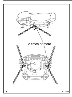
(3) Using 3 wire harness, wind the wire harness at least 2 times each around the bolts installed on the left and right sides of the steering wheel pad.
