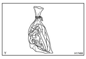
(g) Dispose of the steering wheel pad (with airbag).
