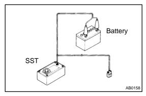
Connect the red clip of the SST to the battery positive (+) terminal and the black clip to the battery negative (-) terminal.
