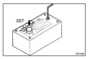
(2) Press the SST activation switch, and check that the LED of the SST activation switch lights up.
