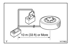
(2) Move the SST to at least 10 m (33 ft) away from the steering wheel pad tied down on the disc wheel.
