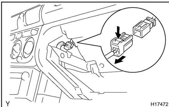
(b) Disconnect the airbag connector.
