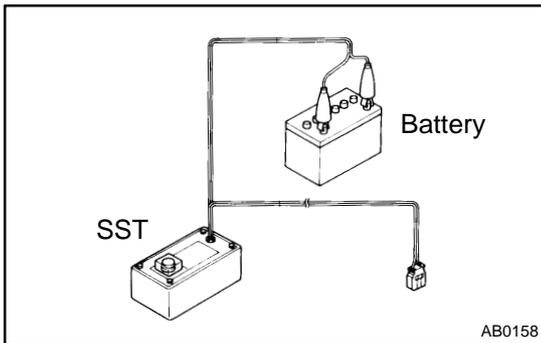
(1) Connect the SST to the battery.
