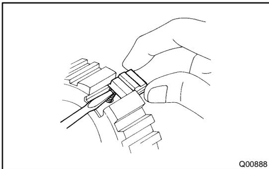
**2. INSTALL CLUTCH HUB NO.1 INTO REVERSE GEAR**
