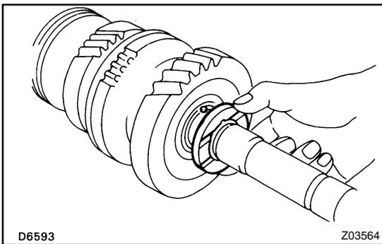
**9. INSTALL STRAIGHT PIN AND 1ST GEAR THRUST WASHER**
