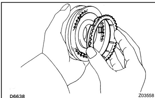
**3. INSTALL 3RD GEAR AND HUB SLEEVE NO.2 ON OUTPUT SHAFT**
