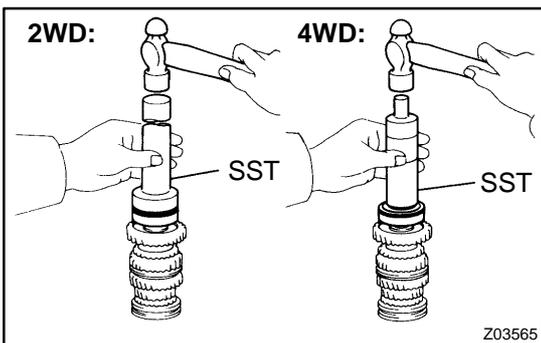
**10. INSTALL OUTPUT SHAFT CENTER BEARING**
