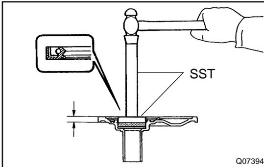
(b) Using SST and a hammer, drive in a new oil seal.
