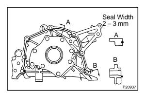
(b) Apply seal packing to the oil pump, as shown in the illustration.
