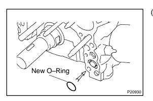
(c) Place a new O-ring into the groove of the cylinder block.
