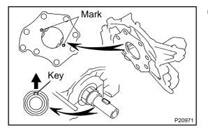
(d) Install the oil pump to the crankshaft with the spline teeth of the drive rotor engaged with the large teeth of the crankshaft.
