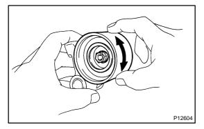
(b) Check that the idler pulley turns smoothly. If necessary, replace the idler pulley.
