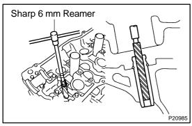
(h) Using a sharp 6 mm reamer, ream the guide bushing to obtain the standard specified clearance (See page EM-38) between the guide bushing and valve stem.
