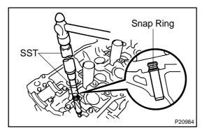
(g) Using SST and a hammer, tap in a new guide bushing until the snap ring makes contact with the cylinder head.
