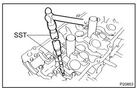
(c) Using SST and a hammer, tap out the guide bushing. SST 09201–10000 (09201–01060), 09950–70010 (09951–07150)
