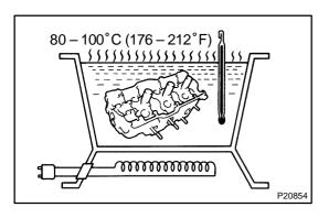
(b) Gradually heat the cylinder head to 80 – 100°C (176 – 212°F).
