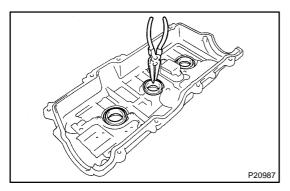
(c) Using needle-nose pliers, pry out the gasket.
