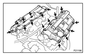
23. REMOVE EXHAUST MANIFOLDS
