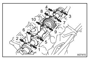
(b) Remove the intake camshaft of the RH cylinder head.
