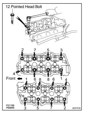
(c) Uniformly loosen and remove the 8 cylinder head (12 pointed head) bolts on each cylinder head, in several passes, in the sequence shown, then repeat for the other side, as shown. Remove the 16 cylinder head bolts and plate washers.
