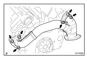
**22. REMOVE EXHAUST CROSSOVER PIPE** Remove the 6 nuts, crossover pipe and 2 gaskets.
