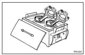
(b) Gradually heat the piston to about  $60^{\circ}C (140^{\circ}F)$ .
