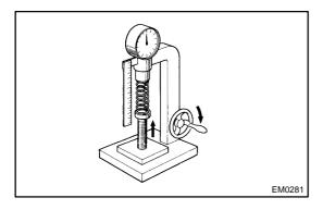
(b) Using a spring tester, measure the tension of the valve spring at the specified installed length.
