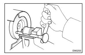
(e) Check the surface of the valve stem tip for wear. If the valve stem tip is worn, resurface the tip with a grinder or replace the valve.
