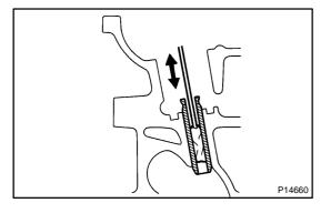
(c) Using a valve guide bushing brush and solvent, clean all the guide bushings.
