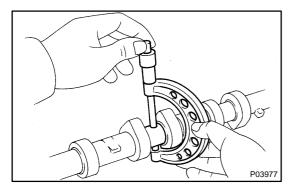
(c) Using a micrometer, measure the journal diameter.
