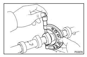
(b) Using a micrometer, measure the cam lobe height. Standard cam lobe height:
