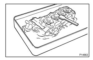
(d) Using a soft brush and solvent, thoroughly clean the cylinder head.
