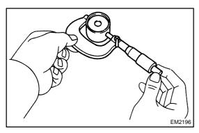
(b) Using a micrometer, measure the lifter diameter.
