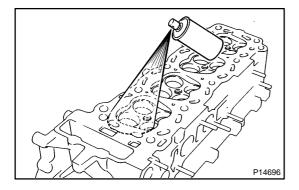
(b) Inspect for cracks.
