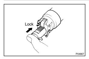
(b) Released the ratchet pawl and check that the plunger is locked in place by the ratchet pawl and does not move when pushed with your finger.
