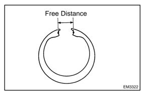
(d) Using a vernier caliper, measure the free distance between the gear spring ends.
