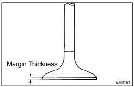
(c) Check the valve head margin thickness.
