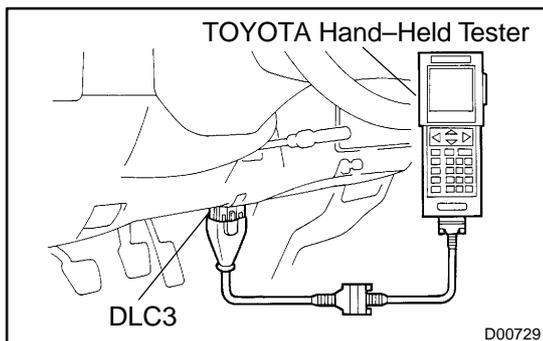
**6. DTC CLEARANCE (Using hand-held tester)**
