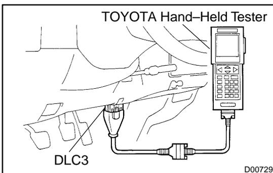
**3. DTC CHECK (Using hand-held tester)**
