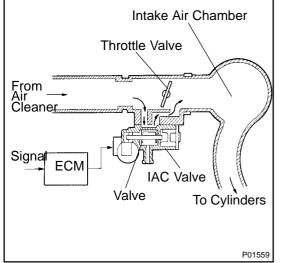
The rotary solenoid type IAC valve is located in front of the intake air chamber and intake air bypassing the throttle valve is directed to the IAC valve through a passage.
