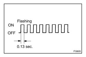
(6) Switch the hand–held tester from the normal mode to the check mode (check that the MIL flashes).
