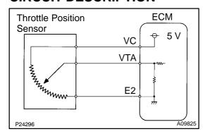
The throttle position sensor is mounted in the throttle body and detects the throttle valve opening angle.
