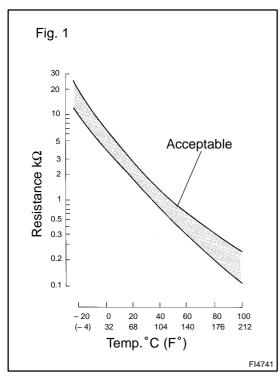
The intake air temperature sensor is built into mass air flow meter and senses the intake air temperature.
