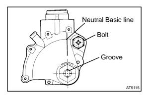
(g) Inspect and adjust the park/neutral position. Check that the engine can be started with the shift lever only in the N or P position, but not in other positions.
