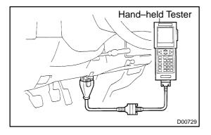
To check the DTCs, connect an OBD II scan tool or hand-held tester to DLC3 on the vehicle. The OBD II scan tool or hand-held tester also enables you to erase the DTCs and check freeze frame data and various forms of engine data (For instruction book). DTCs include SAE controlled codes and Manufacturer controlled codes.
