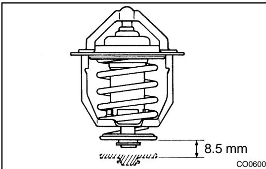
(c) Check the valve lift.
