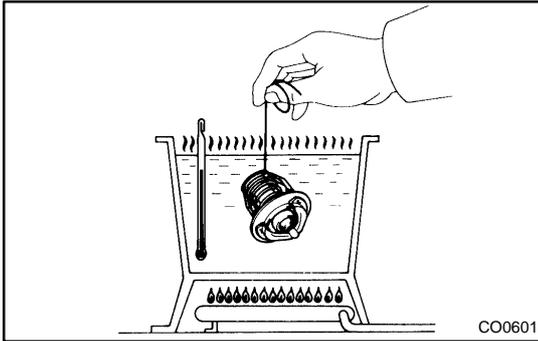
(a) Immerse the thermostat in water and gradually heat the water.
