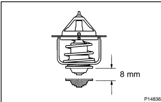
(c) Check the valve opening lift.
