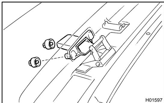
**6. REMOVE REMOVABLE ROOF HINGE CASE**
