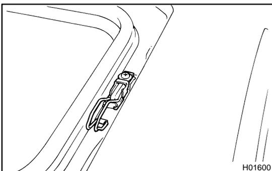
4. REMOVE REMOVABLE ROOF AUXILIARY CATCH
