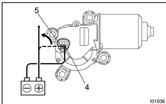
**6. Stopping at Stop Position: INSPECT WIPER MOTOR OPERATION**
