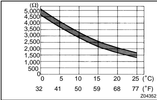
(b) Compare the 2 readings on the chart. If resistance value is not as specified, replace the thermistor.
