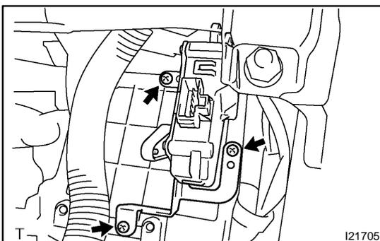
5. INSTALL AIR INLET SERVOMOTOR
