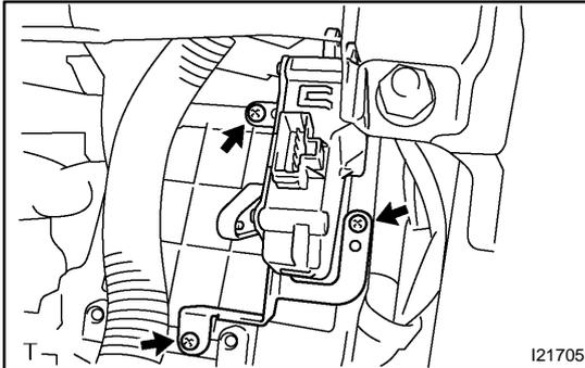
3. REMOVE AIR INLET SERVOMOTOR
