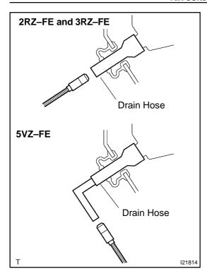
(b) Bring the gas leak detector close to the drain hose before performing the test.
