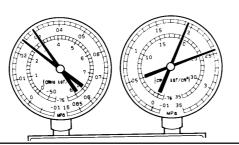
NOTE: These gauge indications are shown when the refrigeration system has been opened and the refrigerant charged without vacuum purging.
