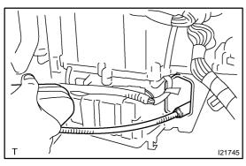
(c) If gas leak is not detected on the drain hose, remove the blower resistor from the cooling unit. Then insert the gas leak detector sensor into the unit and perform the test.
