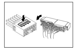
Push the terminal retainer down to the temporary lock position.
