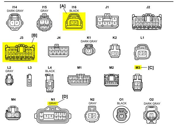
[A]: Indicates connector to be connected to a part. (The numeral indicates the pin No.)
