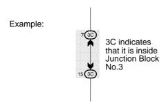
[H]: When 2 parts both use one connector in common, the parts connector name used in the wire routing section is shown in square brackets [ ].
