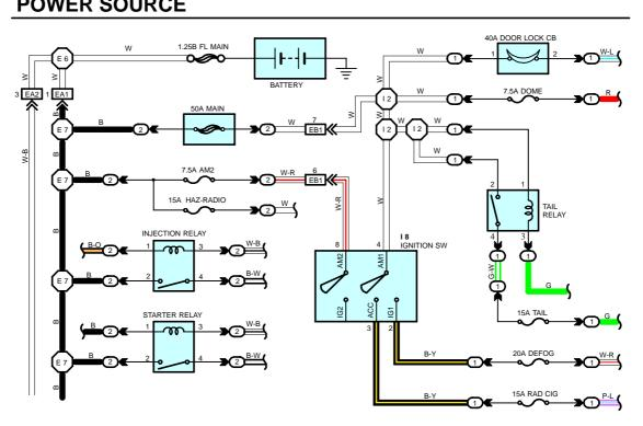
\* The system shown here is an EXAMPLE ONLY. It is different to the actual circuit shown in the SYSTEM CIRCUITS SECTION.
