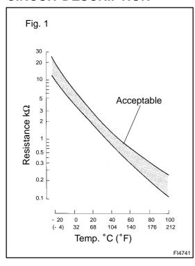
The intake air temperature sensor is built into the mass air flow meter and senses the intake air temperature.
