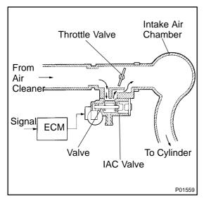
The rotary solenoid type IAC valve is located in front of the intake air chamber and intake air bypassing the throttle valve is directed to the IAC valve through a passage.
