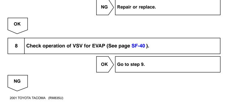
Replace VSV and charcoal canister, and then clean vacuum hoses between throttle body and VSV for EVAP, and VSV for EVAP and charcoal canister.
