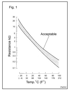
The intake air temperature sensor is Built Into Mass Air Flow Meter and senses the intake air temperature.
