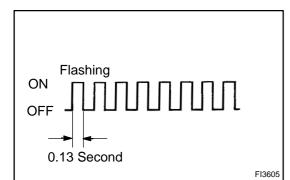
(6) Switch the TOYOTA hand-held tester from the normal mode to the check mode. (Check that the MIL flashes.)
