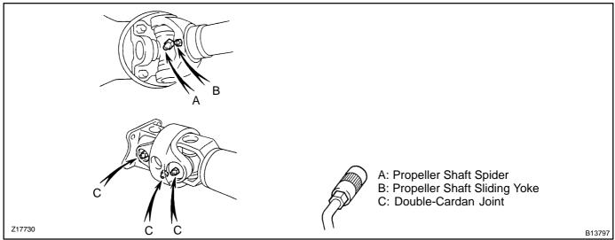
(b) Tighten the bolts for propeller shaft.
